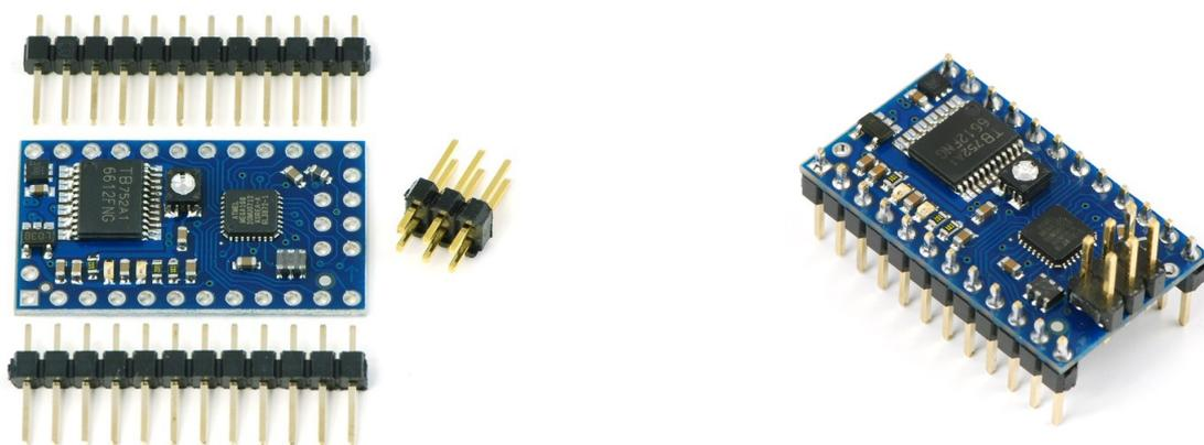
If you solder in the 3×2 ISP header pins, the solder connections should be made along the bottom side of the board so the pin connections are available from the top side of the board, as shown in the right picture above. If you solder the ISP pins to the wrong side of the board, your programmer's ISP cable will not be able to connect correctly to the Baby Orangutan.
